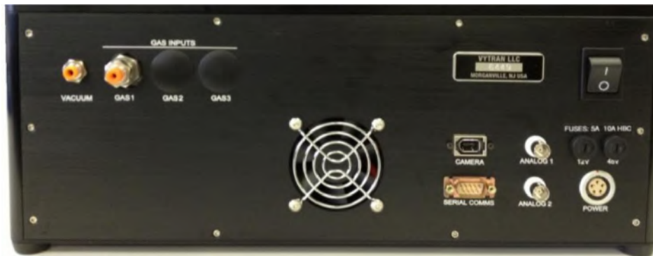
Figure 2 GPX3800 Back Panel Connections
